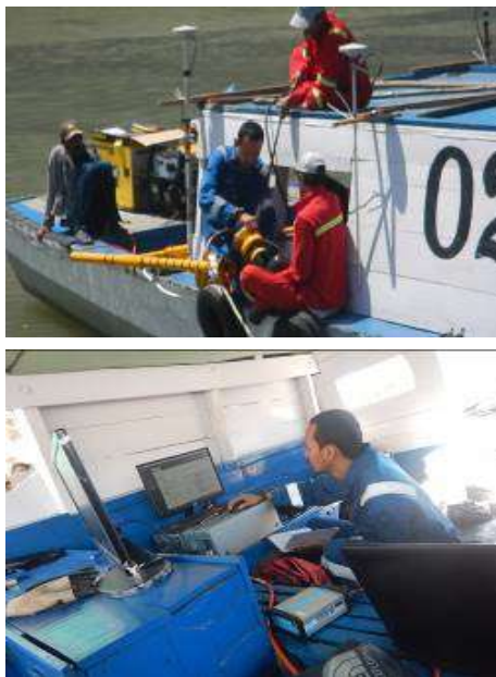
Figure 10: Echo sounder MBES Field Survey.
