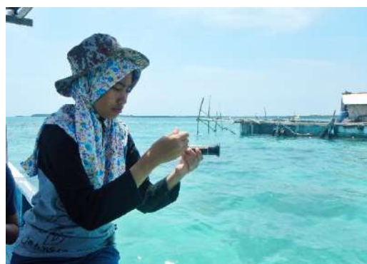
Figure 4: Water Quality Measurement using Refractometer for Salinity.
