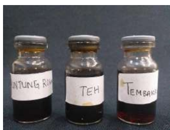
Figure 2: Extraction results of inhibitors from (a) cigarette butt waste (b) tea (c) tobacco.
