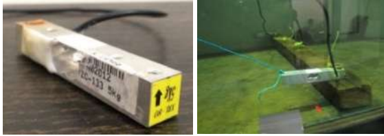
Figure 8: Load Cell with a capacity of 5 kg.
