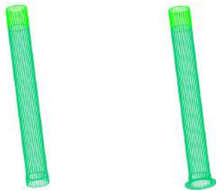
Figure 5: Numerical model of SPAR in MOSES (Full scale) without heave plate (left), and with heave plate (right).
