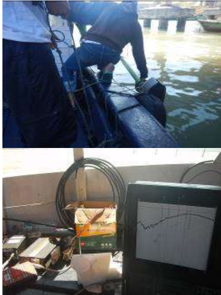
Figure 7: Echo sounder SBES Filed Survey.
