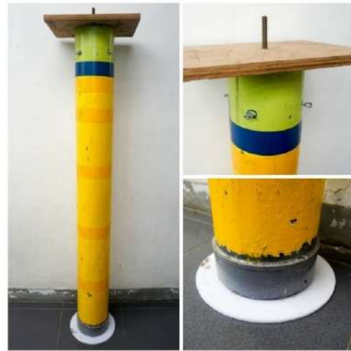
Figure 1: Scale model the SPAR with heave plate.
