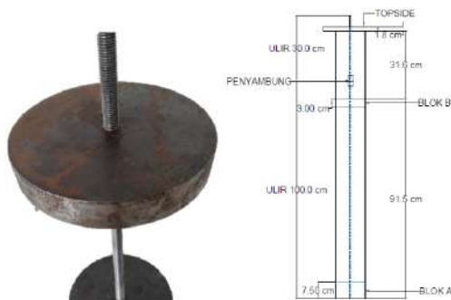
Figure 2: Cylindrical steel as ballast (left) and its configuration inside the SPAR hull (right).
